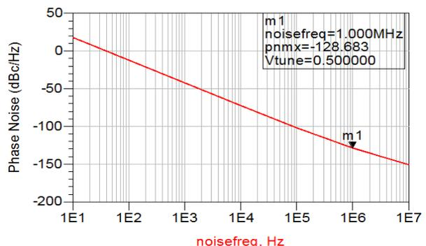
Fig. 5. Phase Noise at 1 MHz Offset
