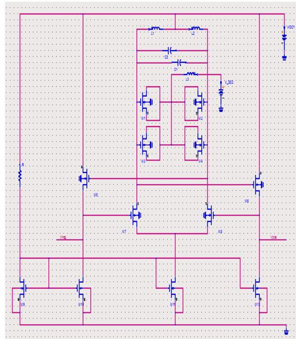
Fig4 Schematic of NMOS Cross-coupled VCO
